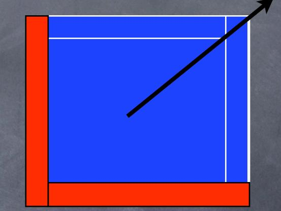
The high concentration tracer coming into the box is **immediately mixed** with the the low concentration tracer left in the box.
